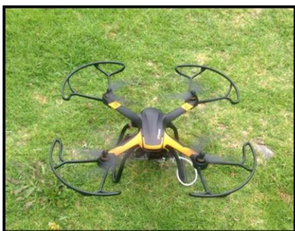
Fig. 12 Hubsan X4 PRO unmanned aerial vehicle equipped with CC and ready to perform flight test
