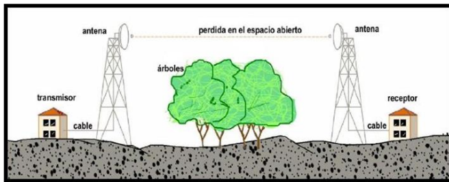
Fig. 4 Microwave terrestrial link between a receiving station and a transmitting station
