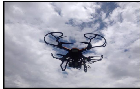
Fig. 13 Hubsan X4 PRO unmanned aerial vehicle equipped with DC during flight
