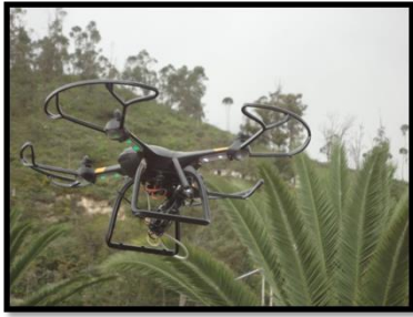
Fig. 15 . Hubsan X4 PRO unmanned aerial vehicle equipped with DC during flight
